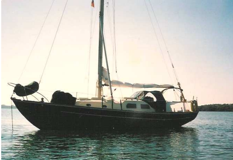
Note the stowed whisker pole, boom gallows and a jib bagged on the forestay
